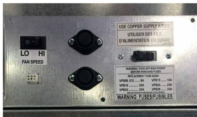
Figure 12: Unit switch plate with ada thermostat connection
